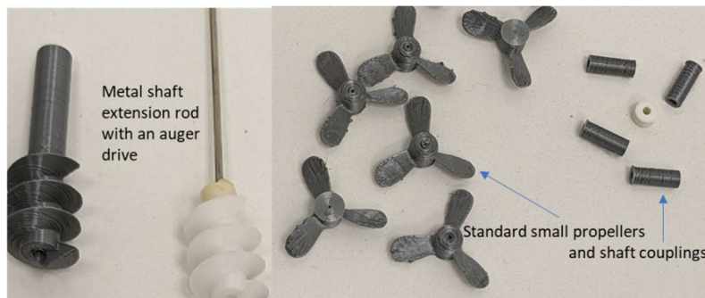
Figure 3 Potential drive elements for connection to motor
